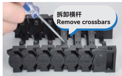
螺丝刀插入槽中利用杠杆运动撬开横杆 Insert screwdriver into the slot. Using a lever action, release the crossbars
