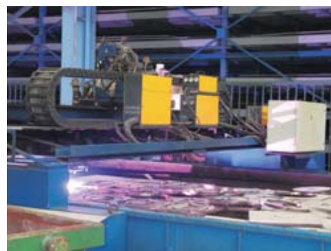
激光切割设备 Laser cutting equipment
