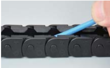
压装电缆 Press in cable
